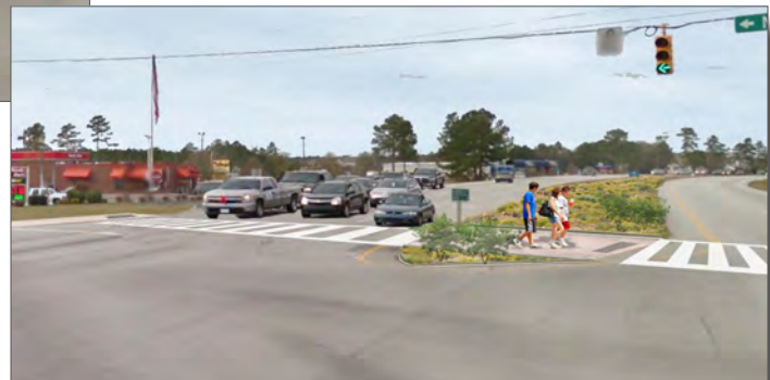
Proposed conceptual improvements include high-visibility crosswalks and a pedestrian refuge island.
